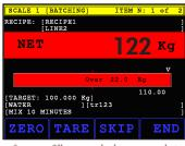
If an overfill occurs the bar goes red. A password protected SKIP button and Cyclic recalculation is then available.
