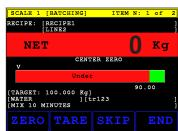
Colour filling bars indicates target weight and tolerances - whilst filling operators aim for the green zone.
