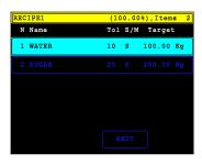
Setting up ingredients, recipes and batch plans is easy via the colour touch screen, QWERTY keypad or PC software. Store and process an almost unlimited amount of products with full traceability and reporting for batches and ingredients. When setting up a product and recipe the following fields are available as standard: Ingredient Name, Code and Batch Code, Recipe Name, Code and Batch Code, Target Weight, Ingredient Tolerances, Recipe Tolerances, Recipe Instructions/Warnings.
